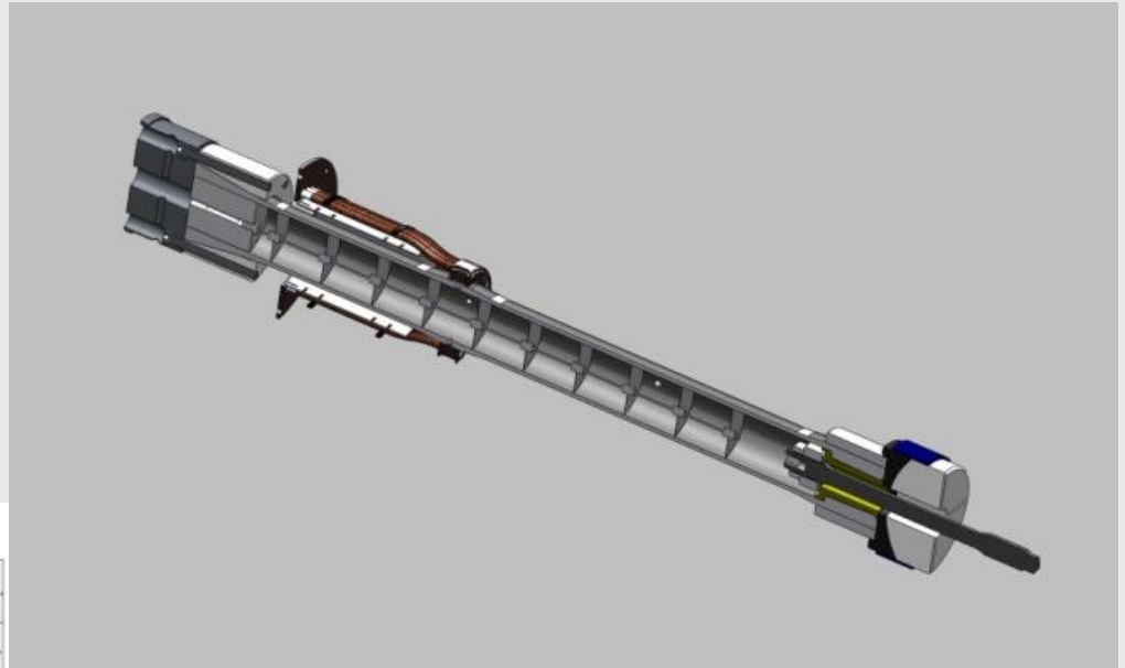
Section Of Composite Compression Tube For Magnet Assembly in MRI Scanners.
